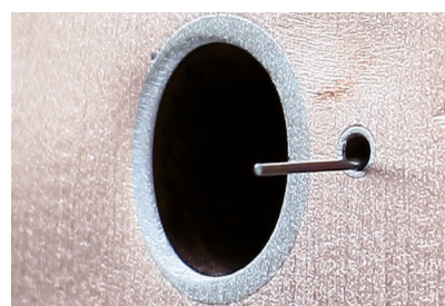
OPTISAVE sensor embedded in cooling block
